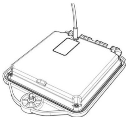
Figure 4.13 Charging the transmitter Li-ion battery pack
