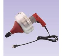
Gorlitz pipe snake GO 31, is our only handheld sink tub drain cleaning machine. Conveniently constructed with a pistol grip, keyless chuck, and trigger action, the 1.60 amp, 120V reversible motor has a variable speed control from 0-450 RPM's to quickly open clogged drains. Enclosed in an aluminum drum holding up to 50 feet of 5/16" cable, this machine cleans drain lines from 11/4" to 2" in diameter up to 50 feet long.
